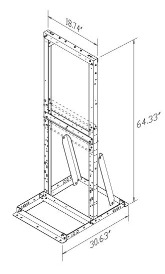
**Description:** Commercial Multi-Rack System (#MR-2) Weight: 48.4 lbs Maximum Capacity: Up to 220.5 lbs / 100.0 kgs Compatibility: All Noritz Commercial Models
